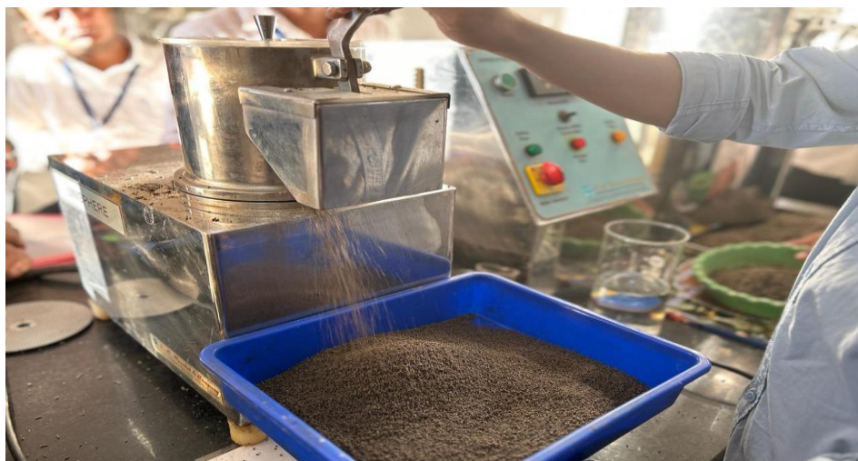
Fig4: Pelleted feed preparation by the trainees using the spheronizer
